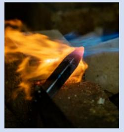
**5.** The punch is heat-treated to harden and temper it.
