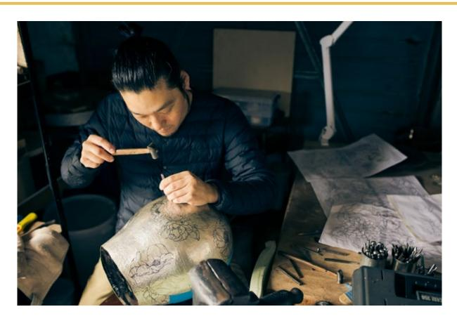
pitch inside a piece with a heat gun – like a strong hairdryer – when he is chasing to make the silver easier to work with.
