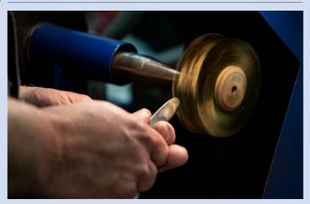
**6.** Once hardened, the punch is brushed back with a brass brush to clean fire stains. Then the punch is given its final inspection.
